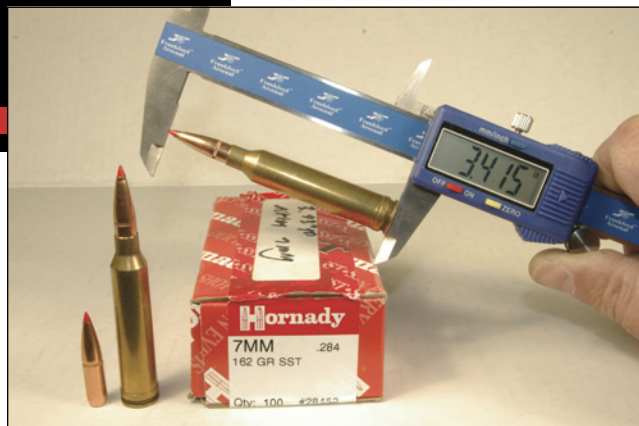
Seating depth can influence accuracy. Finding a sweet spot – how far short a bullet should be from the rifling – often requires experimentation.
