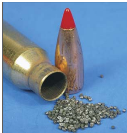
Exact propellant weights help keep velocities constant in the .221. One additional grain of IMR-4227 increased velocity of the Hornady 40-grain V-MAX by more than 200 fps.
